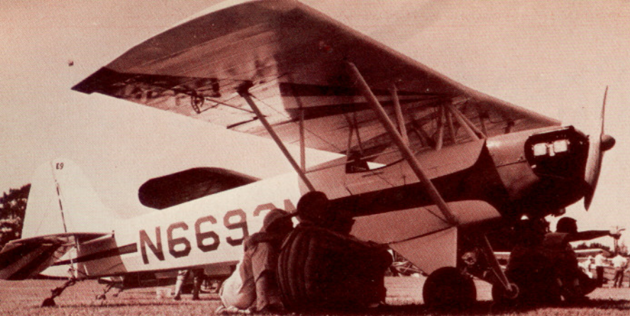
▲ Corben "Baby Ace" was factory design of 1930's, based on the Heath Parasol. Recently redesigned to use more modern components, including Piper Cub landing gear, it is one of the most popular designs available to home builders of aircraft
