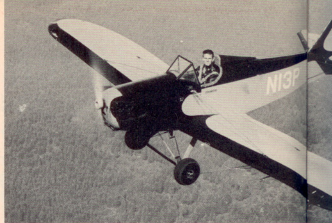
▲ Author Bowers designed the all-wood "Fly Baby" which sacrifices top speed for improved low speed and "over-the-fence" characteristics
